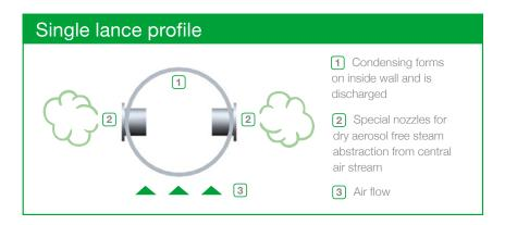
MultiLance systems are simple to install, maintenance-free and the high quality stainless steel components afford a long lifetime. Thanks to the special nozzle format the steam is obtained without aerosols from the middle of the lance, so that the downstream sensitive duct installations can be effectively protected from condensation.
