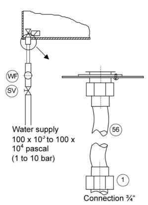
» HygroMatik provides a water hose (56) with a cap nut at both ends which can be used for water installation.
