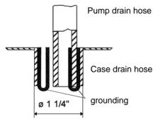
2 grounding clips are fixed on the inner surface of the housing drain connection. During blow-down, the grounding clip is in direct contact with the water and shunts potential residual electric currents away from the housing.
