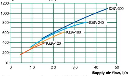
The diagram shows the approximate cooling effect  $P_{tot}$  in W with water flow  $q_w = 0.05$  /s, temperature difference between room air and supply air  $\Delta t = 8$  °C, difference between room air and average water temperature = 8 °C, pressure drop 60 Pa on the air side and max. sound pressure level  $L_{A10} = 34$  dB(A).
