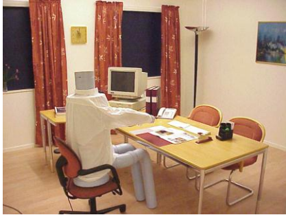
Large office room - cooling coil-CAV - Air flow 20 l/s - Cooling capacity 1150 W
