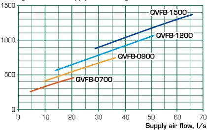
The diagram shows the approximate cooling effect,  $p_{tot}$  in W with a water flow of = 0.05 l/s, temperature difference between supply air and room temperature,  $\Delta t$  = 8 °C and an operating pressure of 200 Pa.
